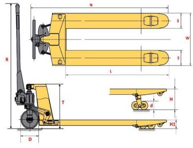
With dimensions over the forks of **540x1150mm**, this is the ideal size for the most common **Euro Pallets of 120x80cm**, but will also lift the common **GKN/Chep pallets of 120x100cm** and many other sizes.
