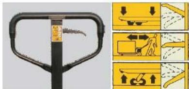
**Lower Position** - to lower load, pull up on the finger tip control.
