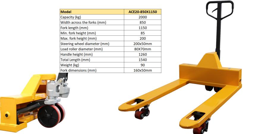
A very specialised pallet truck, this extra wide hand pallet truck has a non-standard fork diameter making it ideal for many special applications. It has a 2000kg capacity, double PU load rollers and steer wheels, pallet entry wheels, durable powered coated main frame and reliable high quality hydraulic pump. The gap between the forks is 530mm
