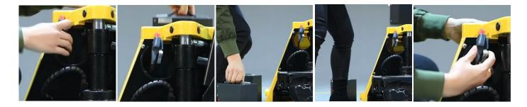
Rated at 2000kg capacity and a slope/climbing gradeability of 6% laden, 20% unladen—this is a powerful machine with average life 3 times greater than a manual pallet truck. Despite this, it's a compact unit, only 32mm longer than a standard pallet truck. Unladen speed is 5km/h and Laden speed 4kh/h.
