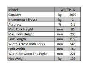
WSPTP1A is a pallet truck with weighing and printing facility
